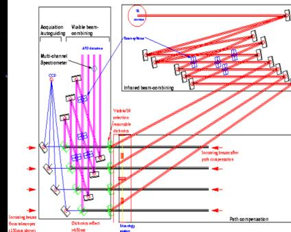
Light from the siderostats enters the bunker. It is then processed as shown.
